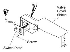
Figure 17 - Installing Switch Plate to Valve Cover Shield
